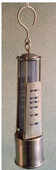
A replica Davy lamp with apertures for measuring flame height
